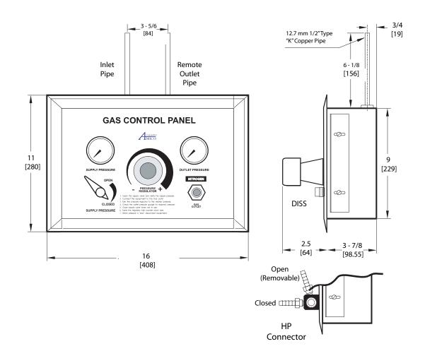
**N-X-CON-ADA-B25** = High pressure adapter with 1/4" Hose barb. (supplied with HP Gas Control Panel).
