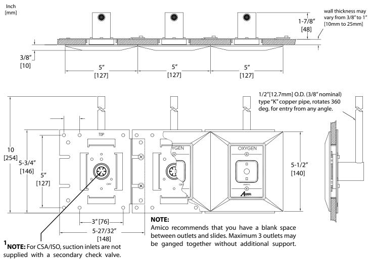
**NOTE:** For CSA/ISO, suction inlets are not supplied with a secondary check valve. A pressure plug is provided for testing purposes, rated at 150 psi [1,034 kPa].
