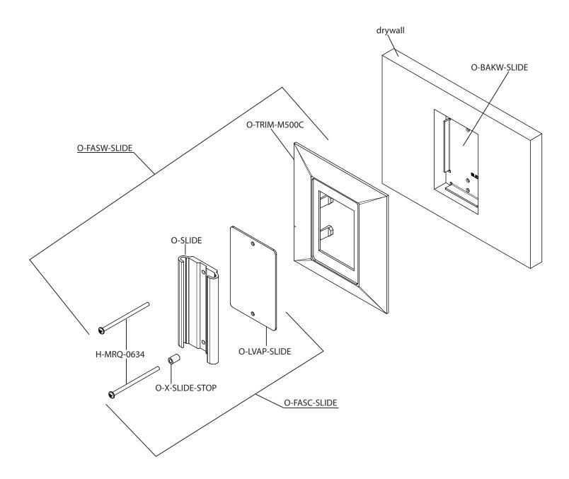
**NOTE:** before installing the bottom screw and slide stopper. Remove and discard the black O-ring.
